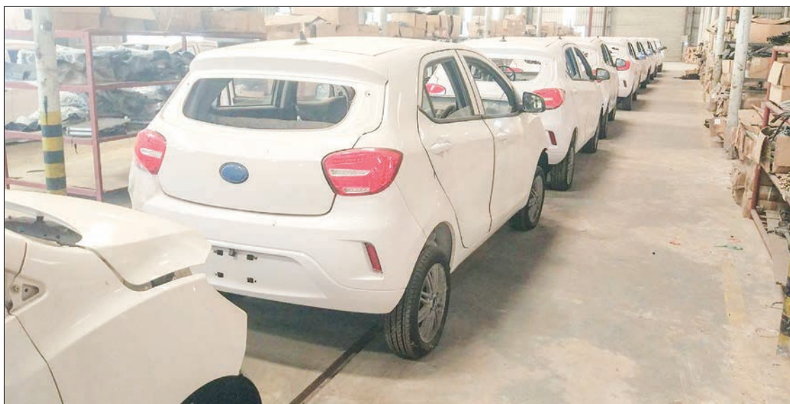
The KSDV 1-NE2 model electric car can drive up to 800 kilometres on a single charge. It can reach speeds of up to 80 kilometres per hour and can have seats of five people. PHOTO: SOE MYINT AUNG
