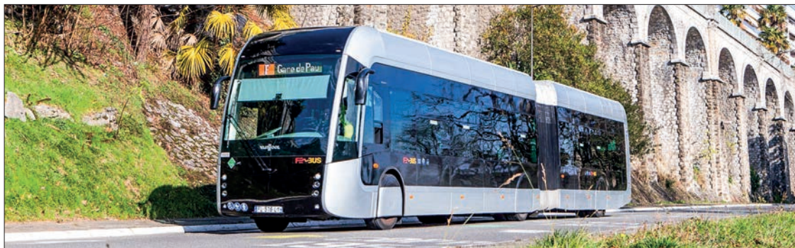
The Pau project will have the first bus line in the world equipped with 18-metre vehicles equipped with a hydrogen fuel cell engine. The new Febus hydrogen bus during its presentation in Pau, France. PHOTO: SNCF/AFP
