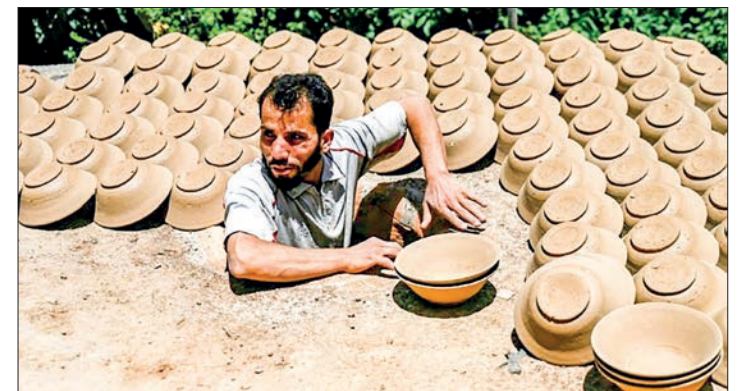
An Afghan potter takes sun-dried bowls from the roof of his kiln to stack for firing in Istalif village, Afghanistan. PHOTO: AFP
