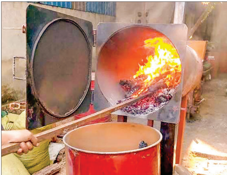
The photo shows the charcoal powder-making machine from husk and sawdust.
