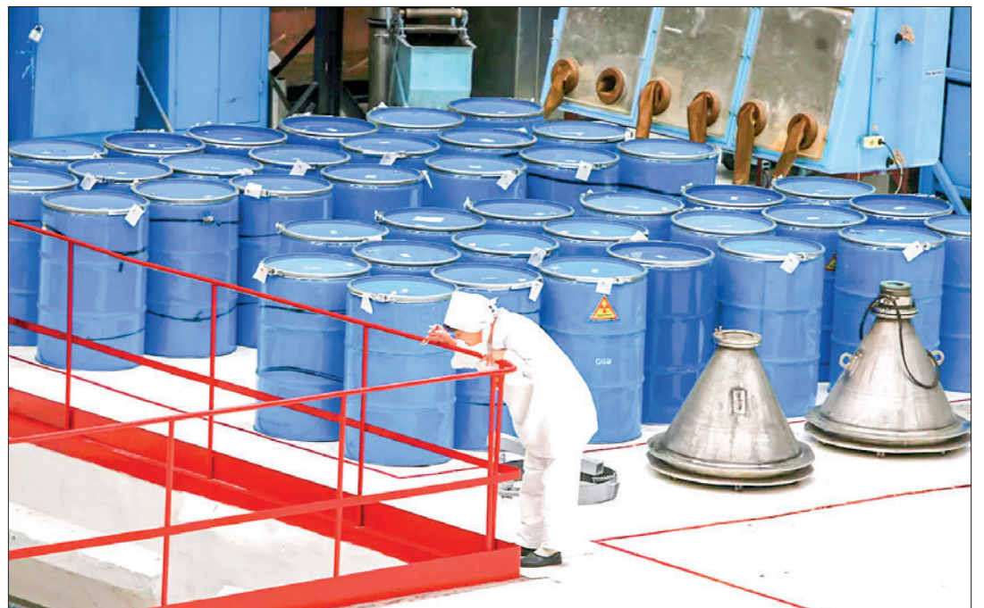
Starting material containers for uranium dioxide fuel pellet production at the Novosibirsk Chemical Concentrate Works. PHOTO: RIA NOVOSTI/SPUTNIK
