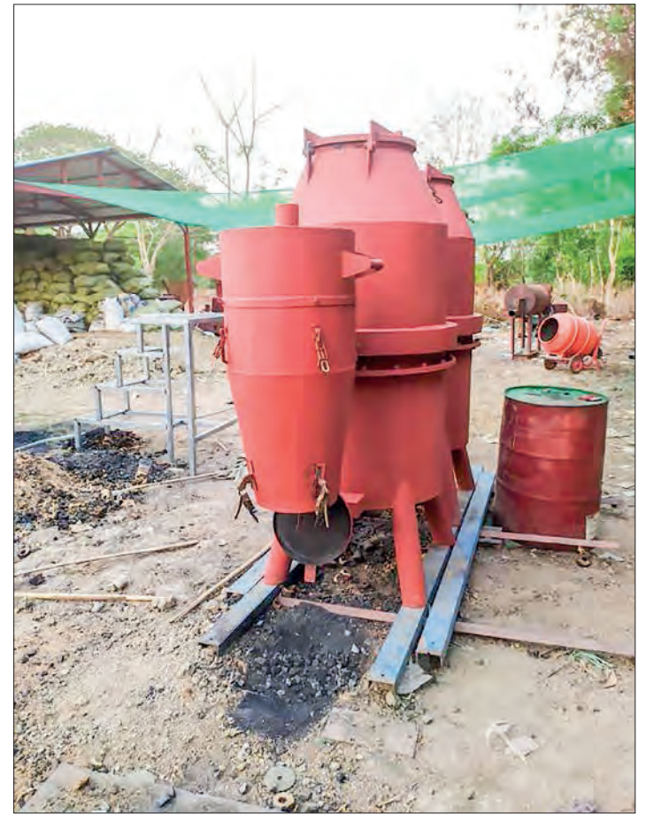
Diesel-substitute paddy husk gasifier that can be used for a 550kW generator invented by a local industrialist.
